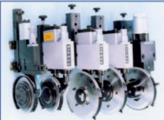
sliding members will wear significantly over time. Excessive wear generated holder looseness changes the shear angle and cut point with detrimental effects to slit quality.
