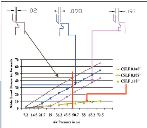
The above graph shows the side load differences for one model top knife holder when the horizontal stroke starting location varies. As can be seen, the closer the blade is to bottom knife, the higher the side load force will be. This is a major factor relative to knife cutting life inconsistencies.
