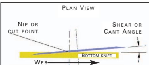
Shear Angle Geometry
